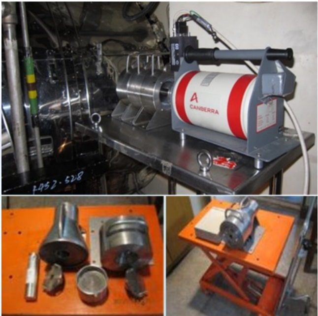
HPGe detector-based \gamma radiation source term measurement system
