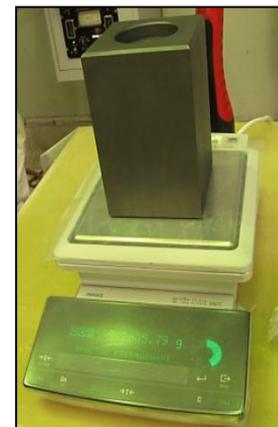
Accepting of the experimental graphite blocks of IGR reactor impregnated by low-enriched uranium
